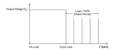
Additionally, if the lo is <135% but >110% for a prolong period of time (depending on the load), the Over Temperature Protection (OTP) will be activated due to high temperature on critical components. The power supply will then go into hiccup mode until the fault is removed; and, the input voltage is removed, then reapplied.
