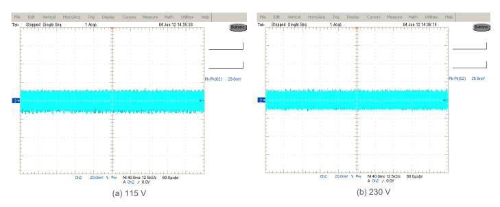
Fig. 2 Ripple & Noise example, 20 MHz BW
