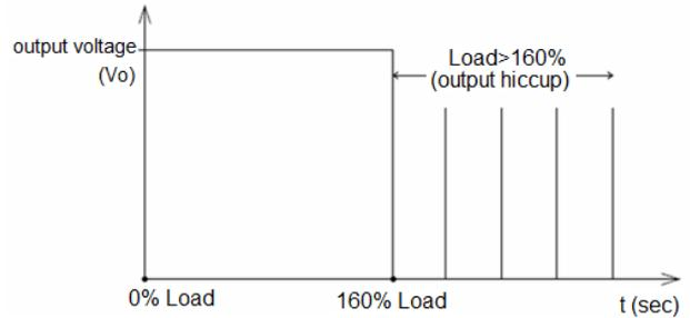
Additionally, if the 48 Volts' lout is  $>100\%$ ; but  $<160\%$  for a prolonged period of time (depending on the load), the Over Temperature Protection (OTP) will be activated due to high temperature on critical components. The power supply will then go into latch mode.
