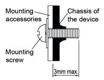
■ For PMT Series (Refer to Fig. 4): Only use M3 screw ≤ 3 mm (0.20 inch) through the base mounting holes. This is to keep a safe distance between the screw and internal components. Recommended mounting tightening torque: 4~7 Kgf.cm.
