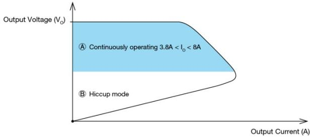
The Overload Protection (OLP) is limited at output power of less than  $100 \text{ W}$  according to safety requirements.
