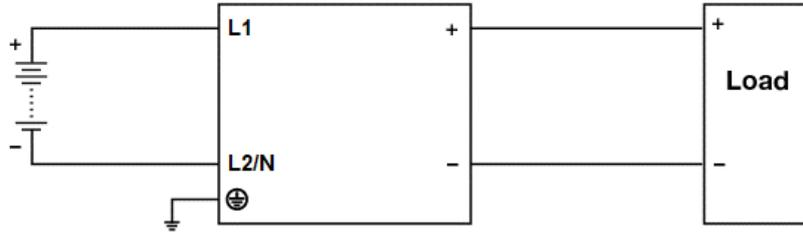
Fig. 6 DC Input Operation Connection Diagram
