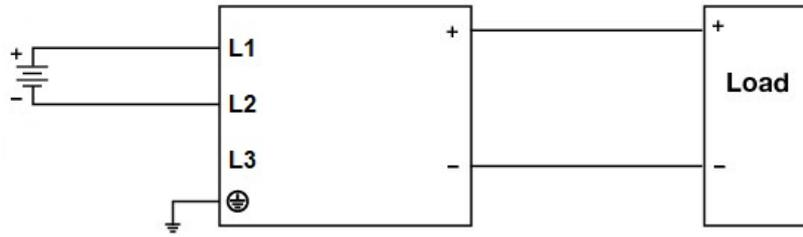
Fig. 7 DC Input Operation Connection Diagram
