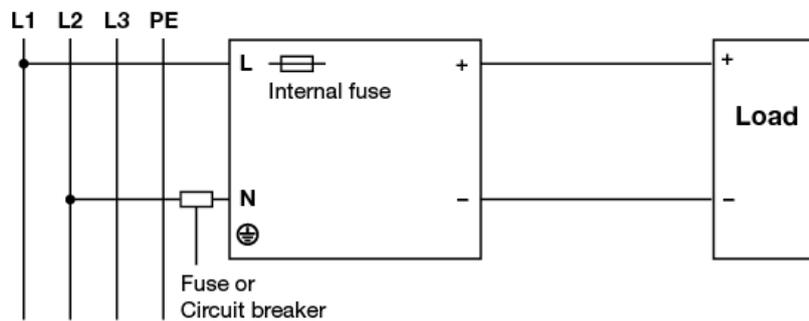
Fig. 9 2 of 3 Phase System Input Operation Connection Diagram
