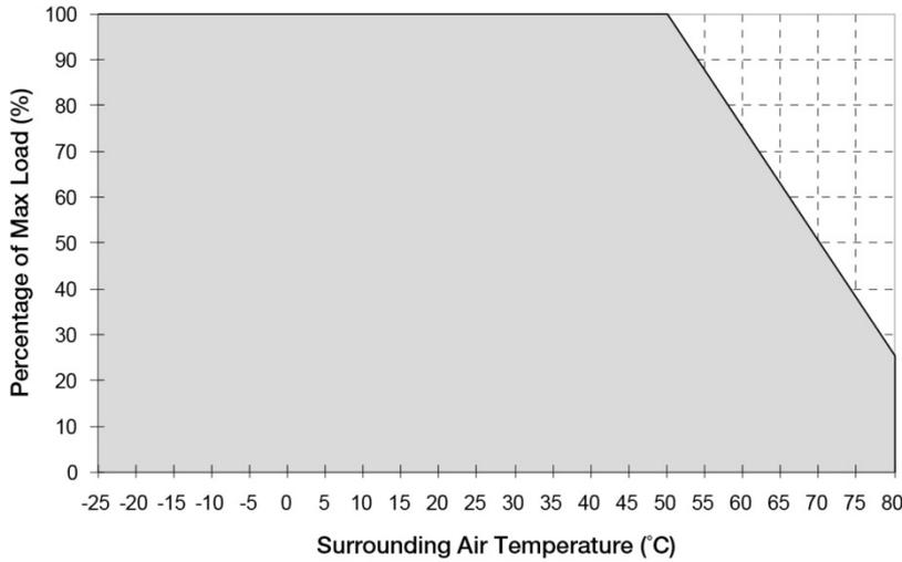
**Fig. 1 De-rating for Vertical and Horizontal Mounting Orientation**
