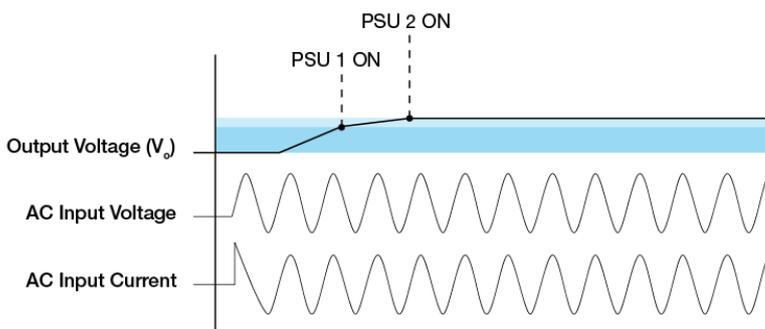
The turn ON would be non-monotonic as the power supply with the fastest startup time and rise time will turn on first. As a result, the startup waveform with 2 power supplies connected in series would see a step.
