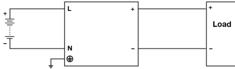
Fig. 8 DC Input Operation Connection Diagram
