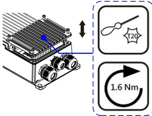
**Note:** The cap and fastening 4 screws all have the function of anti-falling off.
