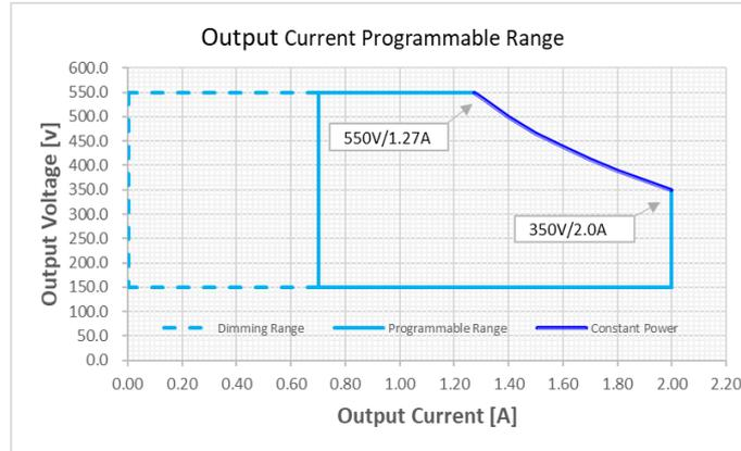
**Note:** EUCO ARENA SPORT 1K4 series can be programmed with wide output current through computer and programming tool. For more details, please refer to DALI programming User Manual or RDM/DMX programming User Manual.
