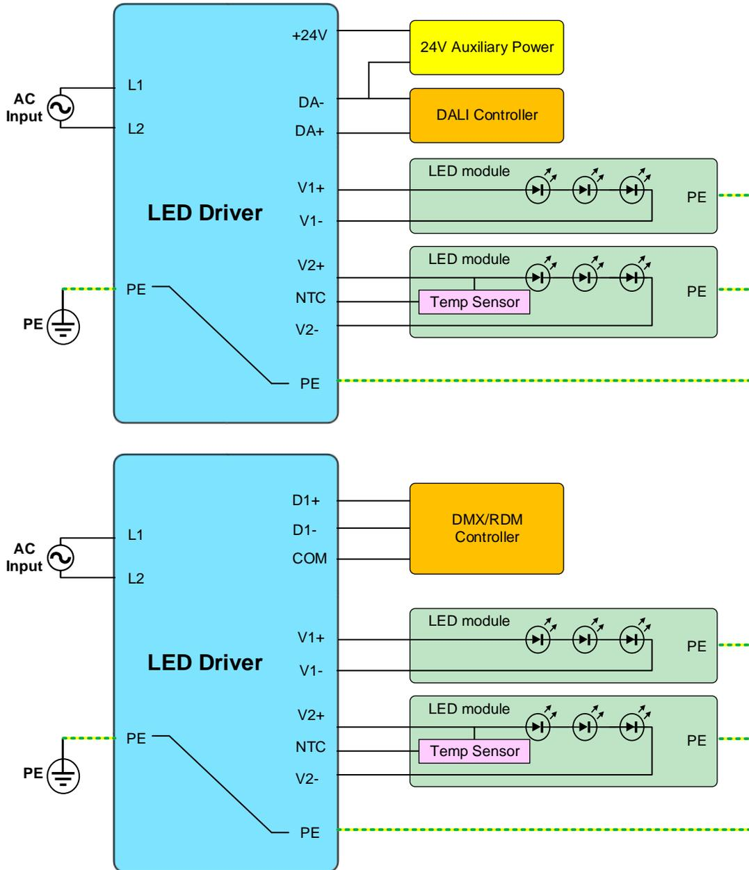
**Note:** All the output channels are independent, any series or parallel connections are not allowed, the user should strictly follow the connection schematic.
