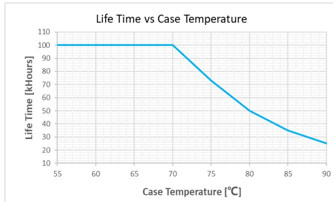
**Note:** Test at input voltage 220Vac & 400Vac, at full Load with each channel 2.0A/350V.
