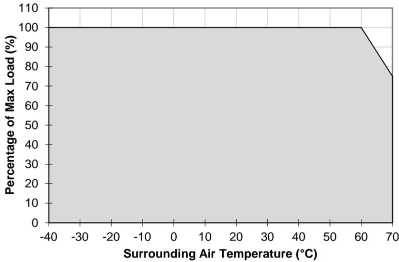
**Fig. 1 De-rating for Vertical Mounting Orientation**
