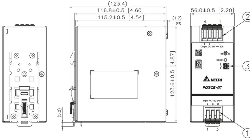
\*Unless otherwise specified tolerance of dimension are ± 0.5 mm
