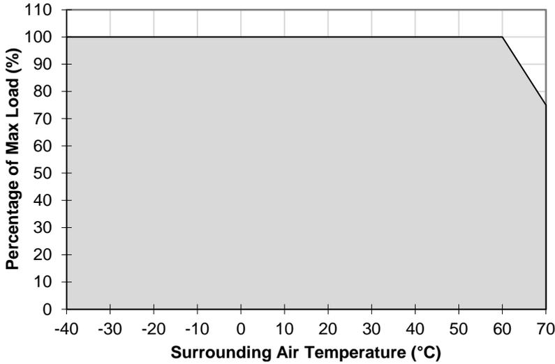
**Fig. 1 De-rating for Vertical Mounting Orientation**
