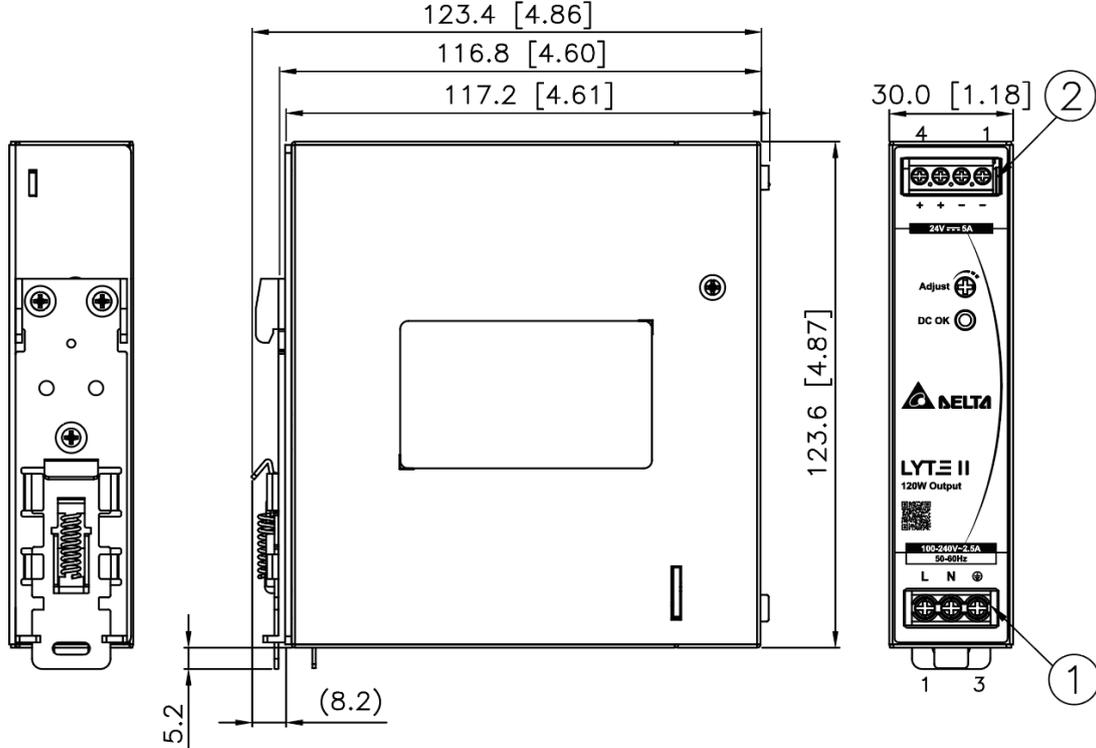
\*Unless otherwise specified tolerance of dimension are  $\pm 0.5$  mm
