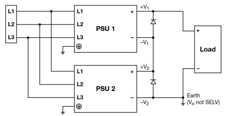
Fig. 11 Series Operation Connection Diagram
