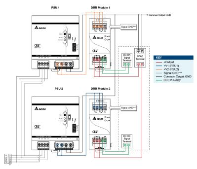
\*\*\*The Signal GND in the DRR module is for the built-in LED and DC OK signals. The Output GND terminals from the two PSU's do not need to be connected to the Signal GND terminal.
