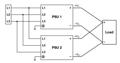
Fig. 10 Parallel Operation Connection Diagram
