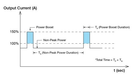
Fig. 7 Duty Cycle Calculation
