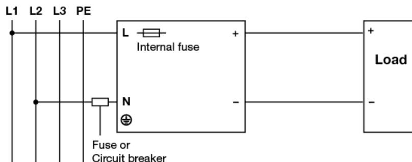
Fig. 7 2 of 3 Phase System Input Operation Connection Diagram
