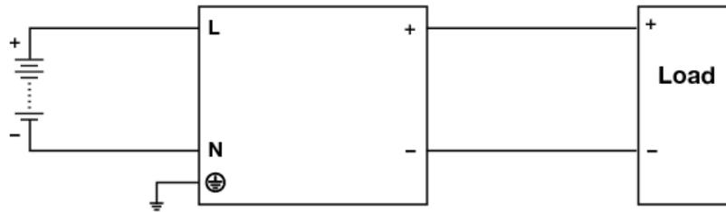
Fig. 6 DC Input Operation Connection Diagram
