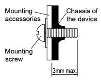
Fig. 4 Mounting Screw
