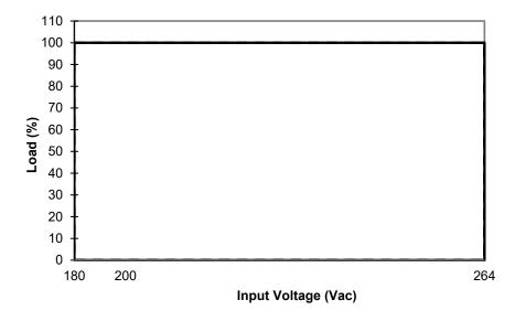
Fig. 2 De-rating for AC Input Voltage
