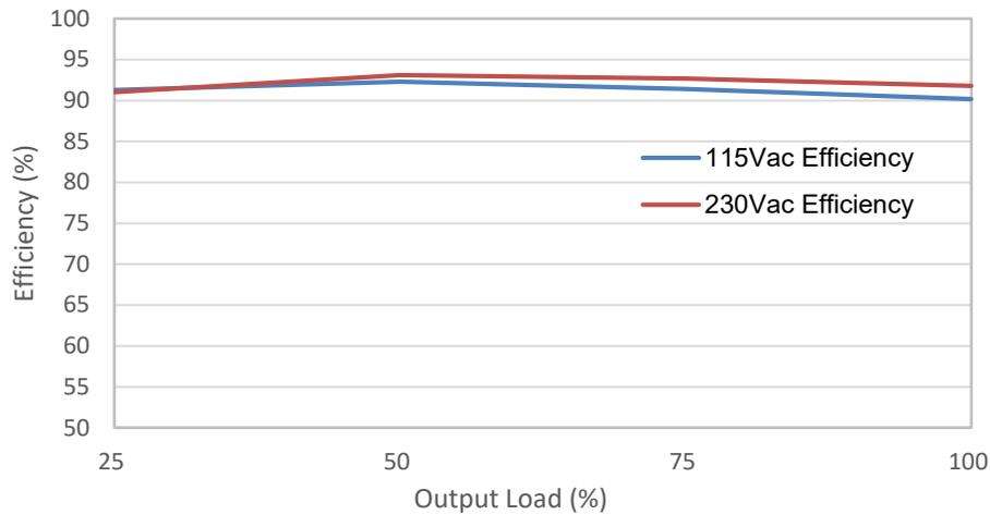
Figure 1. ADT-150A19AA G-A efficiency versus output load
