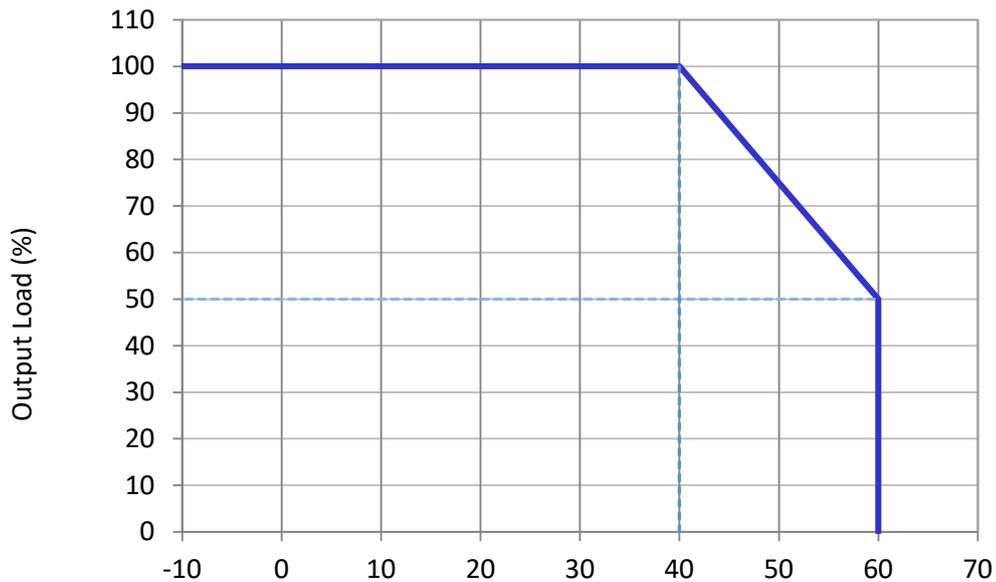
Fig. 1 De-rating for All Mounting Orientation
