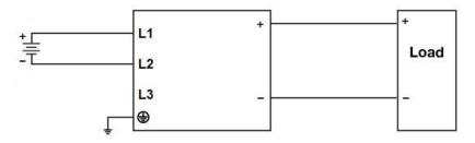
Fig. 5 DC Input Operation Connection Diagram
