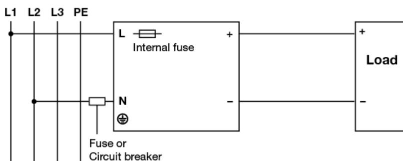
Fig. 13 2 of 3 Phase System Input Operation Connection Diagram
