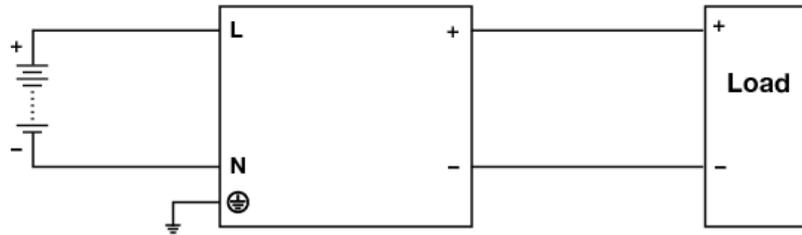
Fig. 6 DC Input Operation Connection Diagram
