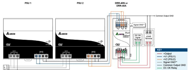
\*\*The Signal GND in the DRR module is for the built-in LED and DC OK signals. The Output GND terminals from the two PSU's do not need to be connected to the Signal GND terminal.
