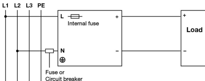
Fig. 13 2 of 3 Phase System Input Operation Connection Diagram
