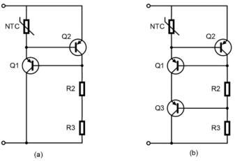
The circuits (a) and (b) have same OTP performance by using the same parts listed in the table, and to achieve good accuracy of OTP, Q2 should be placed close to NTC to make them have same temperature.
