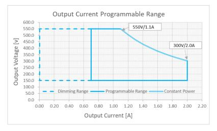
**Note:** EUCO-1K8200GCA series can be programmed with wide output current through computer and programming tool. For more details, please refer to **LNA/EUCO Series Programming Tool User Manual**.
