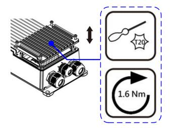
Note: The cap and fastening 4 screws all have the function of anti-falling off.
