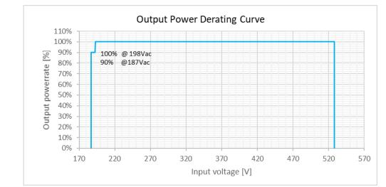
When input range falls from 198Vac to 187Vac<sup>3</sup> the maximum output power would be limited to 1620W by reducing the output current automatically. Hysteresis control logic is applied in triggering/recovering process.
