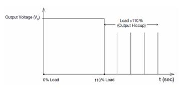
Additionally, if the  $I_0$  is <110% but >100% for a prolong period of time (depending on the load), the Over Temperature Protection (OTP) will be activated due to high temperature on critical components. The power supply will then go into hiccup mode until the fault is removed; and, the input voltage is removed, then reapplied.
