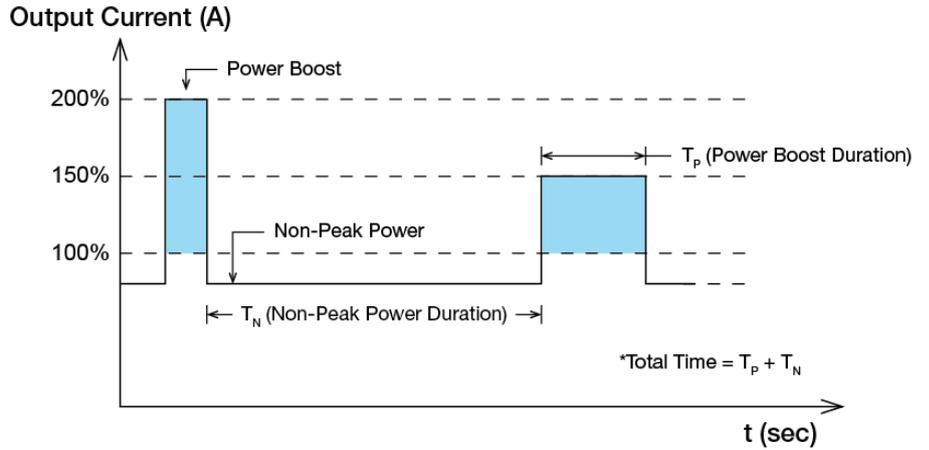
$$\text{Duty cycle (\%)} = \frac{T_P}{\text{Total Time}} ; (T_P \leq 10 \text{ sec})$$
