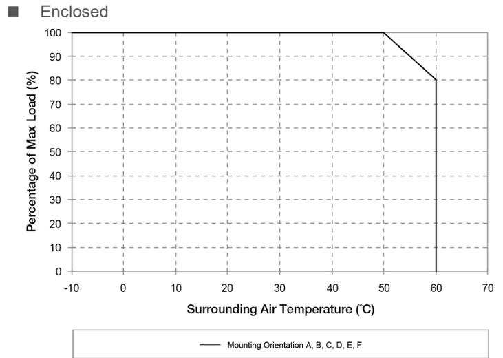
Fig.1.4 De-rating for Mounting Orientation A to F
