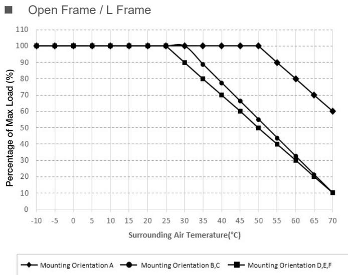
Fig.1.1 De-rating for Mounting Orientation A
