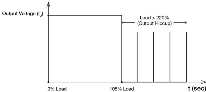
It is not recommended to prolong the duration of  $I_O$  when it is <220% but >100%, since it may cause damage to the PSU.
