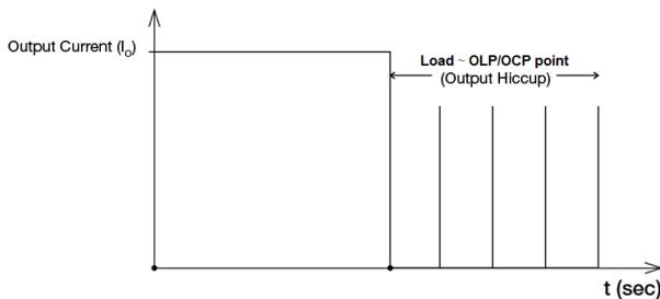
It is not recommended to prolong the duration of I<sub>O</sub> when it is less than OLP/OCP point, but greater than 100%, since such an overload condition may cause damage to the PSU.
