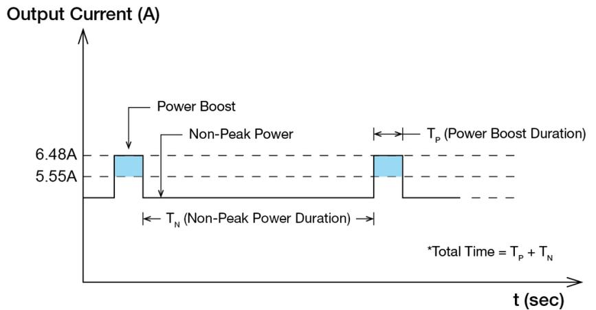
$$\text{Duty cycle (\%)} = \frac{T_p}{\text{Total Time}}$$
