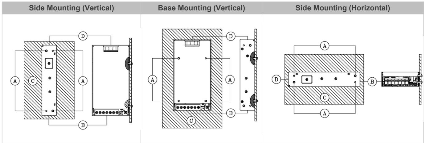
Fig. 2 Mounting Orientation
