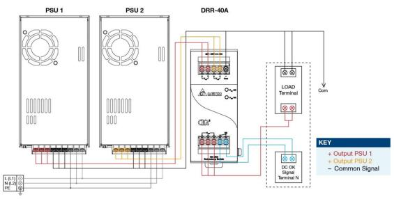
Fig. 5 Redundancy / Parallel Operation Connection Diagram
