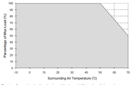
Fig. 1 De-rating for Vertical and Horizontal Mounting Orientation  $> 50^{\circ}C$  de-rate power by 2.5% /  $^{\circ}C$
