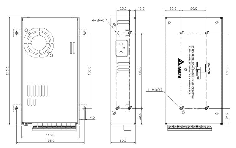
Note : Built-in cooling fan. Must prevent dust suction into power supply, or use natural convection power supply if any concerns.
