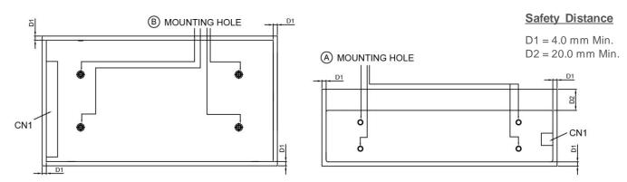
Fig. 3 Mounting Hole Locations and the Safety Distance
