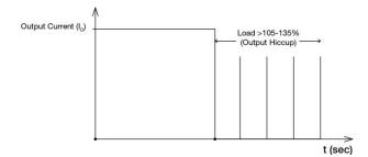
It is not recommended to prolong the duration of  $I_{\rm O}$  when it is <105% but >100%, since it may cause damage to the PSU.
