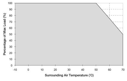
Fig. 1 De-rating for Vertical and Horizontal Mounting Orientation  $> 50^{\circ}$ C de-rate power by 2.5% / °C
