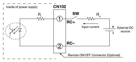
You can remotely control the power supply unit to turn ON/OFF by using an external DC source. Follow the DC power source voltage and current limiting defined in the table below.
