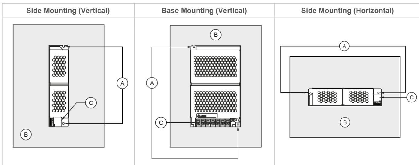
Fig. 2 Mounting Orientation
