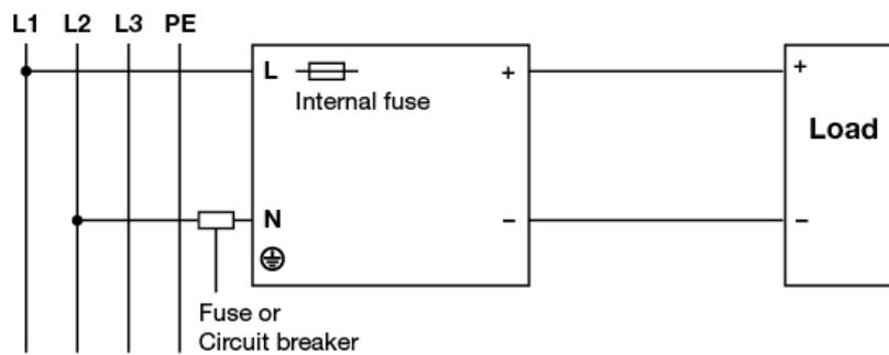
Fig. 6 2 of 3 Phase System Input Operation Connection Diagram
