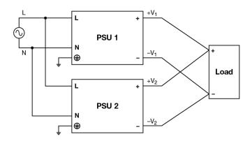
Fig. 6 Parallel Operation Connection Diagram
