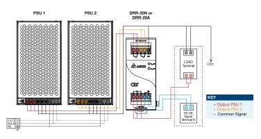
Fig. 5 Redundant Operation Connection Diagram
