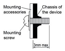
■ For PMT Series (Refer to Fig. 4): Only use M3 screw ≤ 3 mm (0.12 inch) through the base mounting holes. This is to keep a safe distance between the screw and internal components. Recommended mounting tightening torque: 4~7 Kgf.cm (3.47~6.08 lbf.in).
