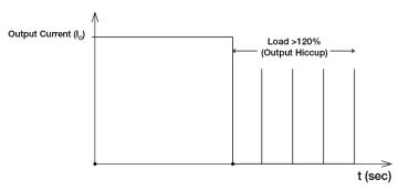
It is not recommended to prolong the duration of I<sub>O</sub> when it is <120% but >100%, since it may cause damage to the PSU.
