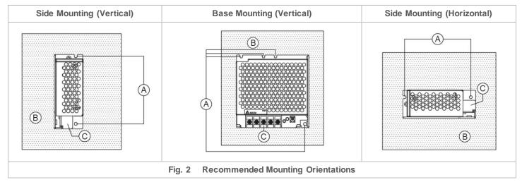
Ensure the mounted device is kept at  $\geq 4\,$  mm (0.16 inch) safety distance at all sides from other components and equipments. In addition, to ensure sufficient convection cooling, always maintain a distance of  $\geq 20\,$  mm (0.79 inch) from ventilated surfaces while the device is in operation.
