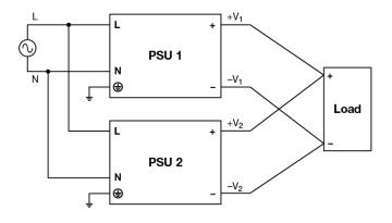
Fig. 6 Parallel Operation Connection Diagram
