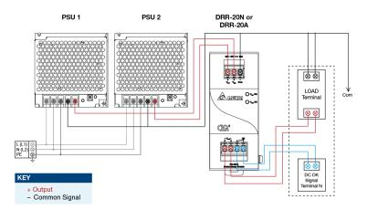
Fig. 5 Redundant Operation Connection Diagram
