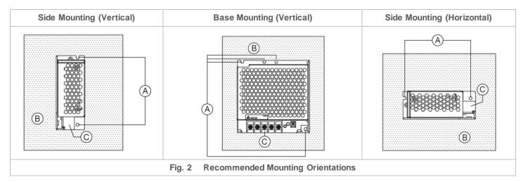
Ensure the mounted device is kept at  $\geq 4 \text{ mm}$  (0.16 inch) safety distance at all sides from other components and equipments. In addition, to ensure sufficient convection cooling, always maintain a distance of  $\geq 20 \text{ mm}$  (0.79 inch) from ventilated surfaces while the device is in operation.
