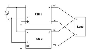
Fig. 6 Parallel Operation Connection Diagram
