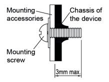
■ For PMT Series (Refer to Fig. 4): Only use M3 screw ≤ 3 mm (0.12 inch) through the base mounting holes. This is to keep a safe distance between the screw and internal components. Recommended mounting tightening torque: 4~7 Kgf.cm (3.47~6.08 lbf.in).
