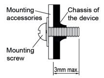
Fig. 4 Mounting Screw
