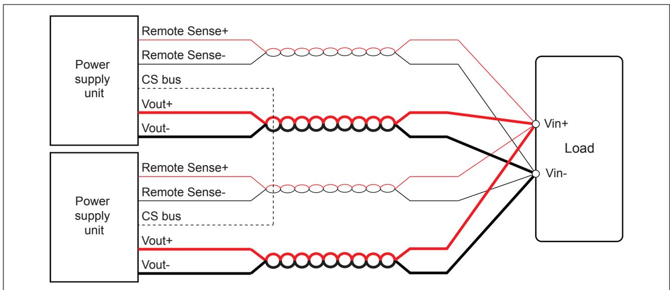
Fig. 15: Active Current Sharing (CS) bus - functional diagram
