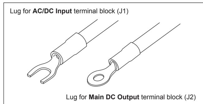
*Fig. 17: Preparing cables for connecting*
