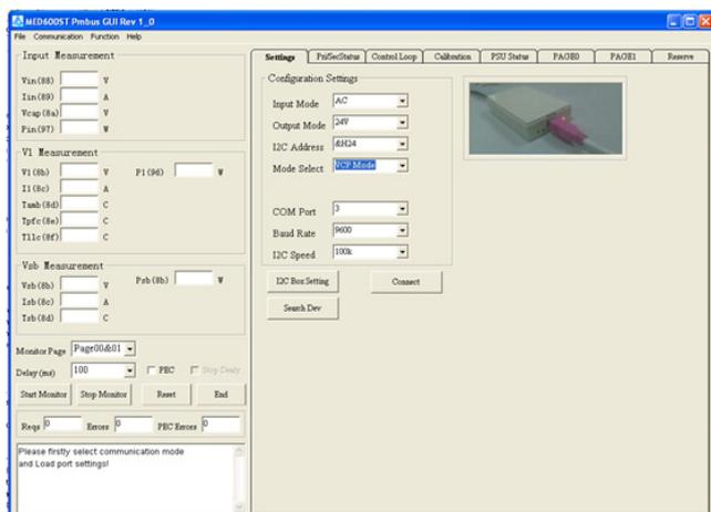
Fig. 34: Graphical User Interface of the PMBus™
