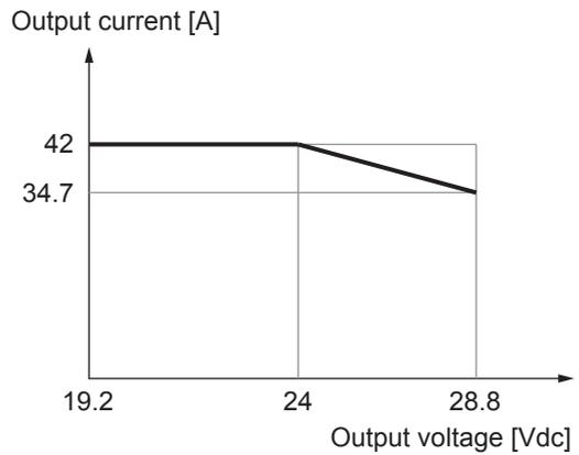
Fig. 29: Output current versus output voltage 24 V
