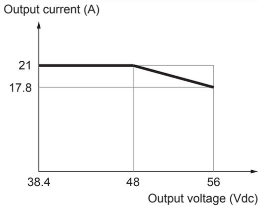
Fig. 30: Output current versus output voltage 48 V
