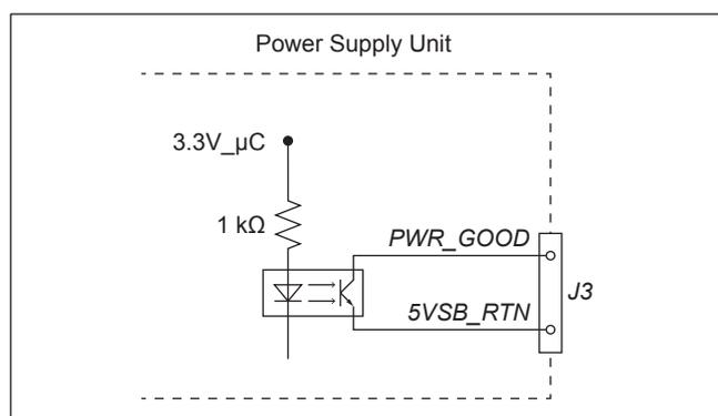
Fig. 12: *PWR\_GOOD* (Power Good) - Circuit diagram
