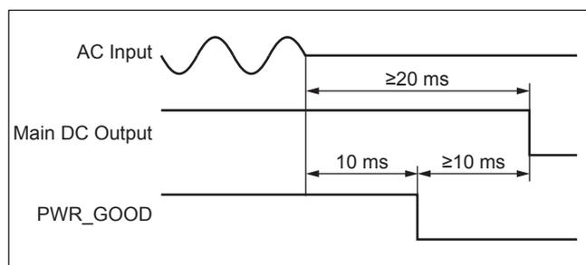
Fig. 13: *PWR\_GOOD* (Power Good) - Signal sequence
