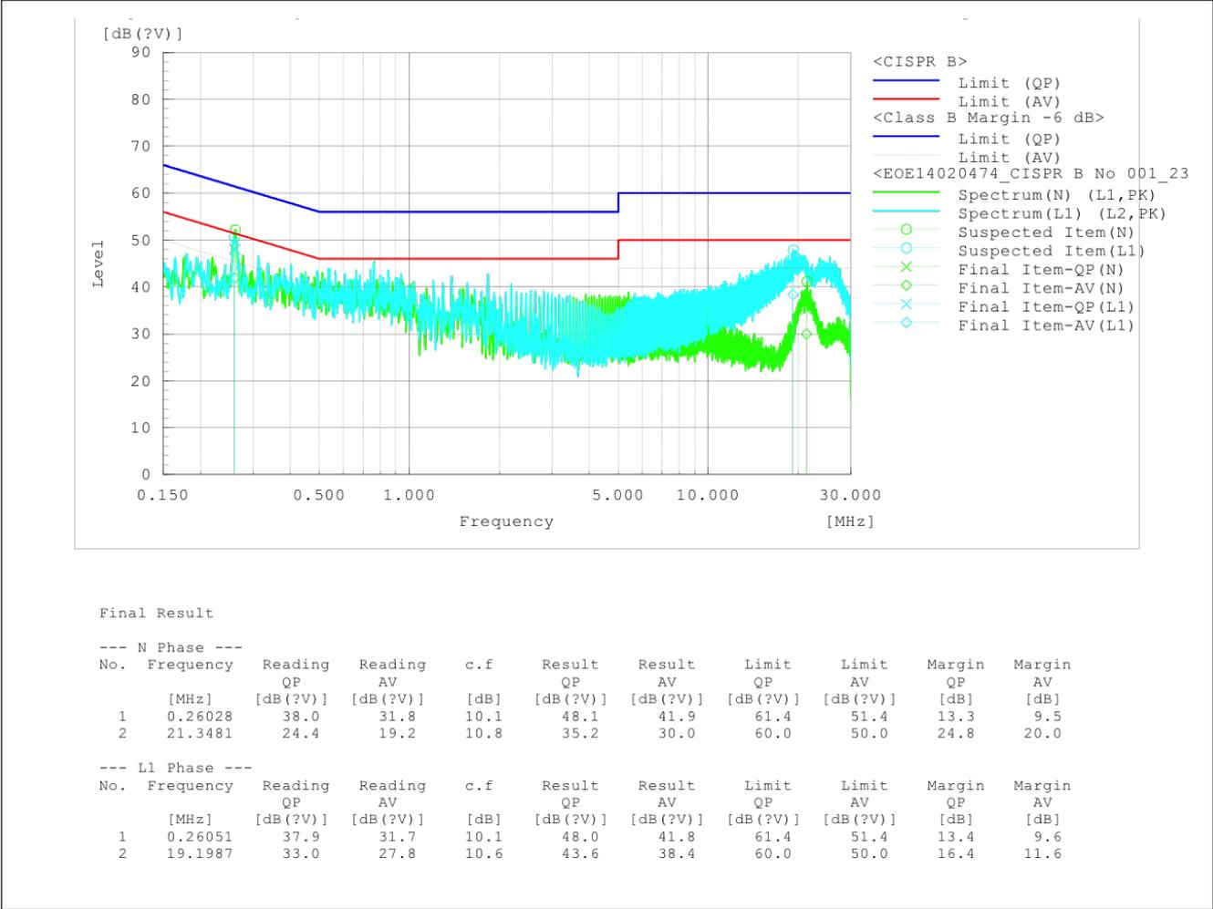
Fig. 18: Electromagnetic compatibility
