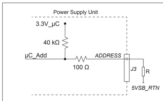
*Fig. 16: Connecting resistor for I<sup>2</sup>C slave address*
