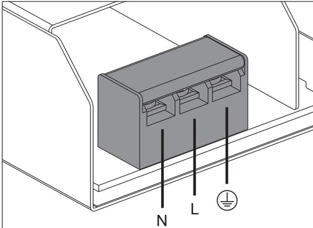
Fig. 2: AC/DC Input terminal block (J1) - pin assignment
