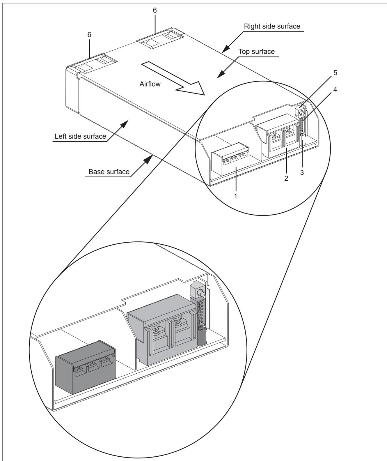
Fig. 1: Components of the IMA-x1000
