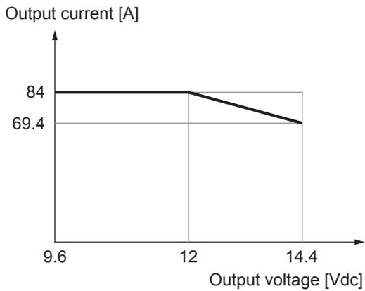
Fig. 28: Output current versus output voltage 12 V
