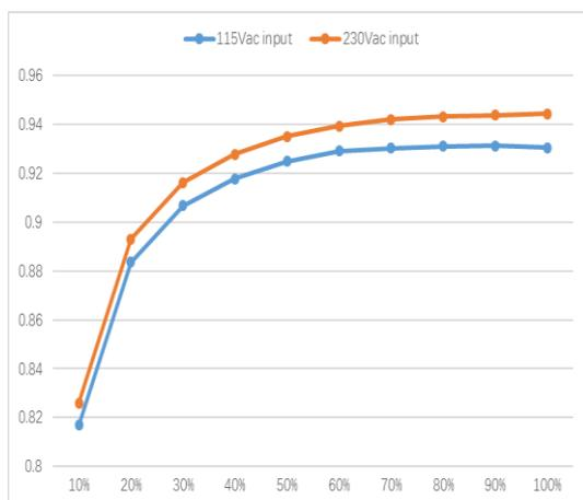
Figure 1. Typical efficiency Curve for 24V (600W max)
