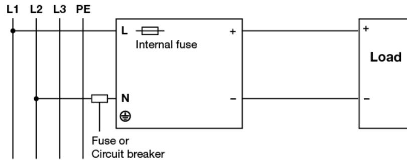
Fig. 5 2 of 3 Phase System Input Operation Connection Diagram
