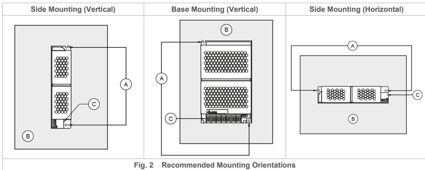
Fig. 2 Recommended Mounting Orientations
