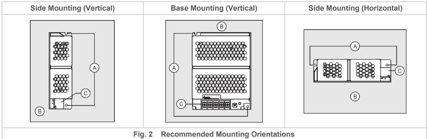
Fig. 2 Recommended Mounting Orientations
