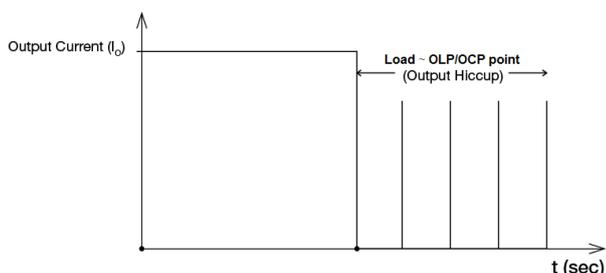
It is not recommended to prolong the duration of  $I_o$  when it is less than OLP/OCP point, but greater than 100%, since it may cause damage to the PSU.
