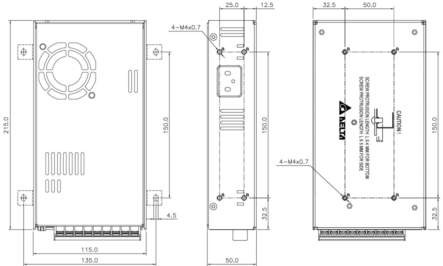
Note : Built-in cooling fan. Must prevent dust suction into power supply, or use natural convection power supply if any concerns.
