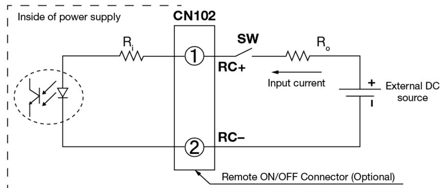
You can remotely control the power supply unit to turn ON/OFF by using an external DC source. Follow the DC power source voltage and current limiting defined in the table below.
