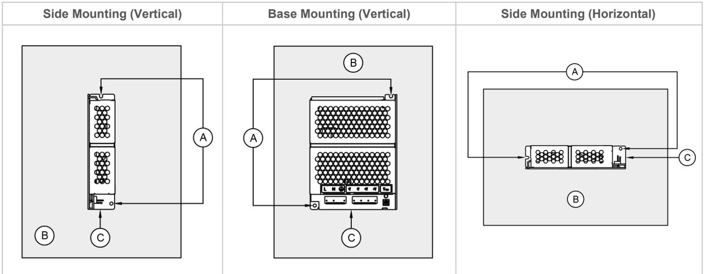
Fig. 2 Mounting Orientation
