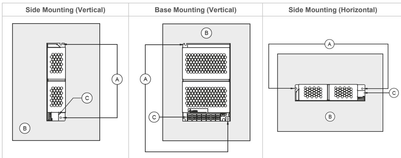
Fig. 2 Mounting Orientation
