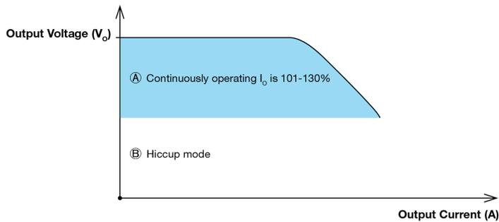
It is not recommended to prolong the duration of  $I_o$  when it is <101~130% but >100%, since it may cause damage to the PSU.
