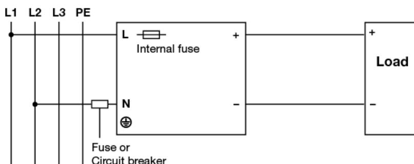
Fig. 6 2 of 3 Phase System Input Operation Connection Diagram
