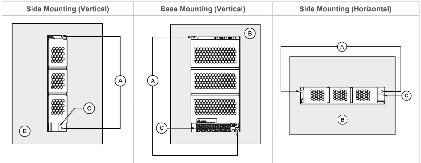
Fig. 2 Mounting Orientation
