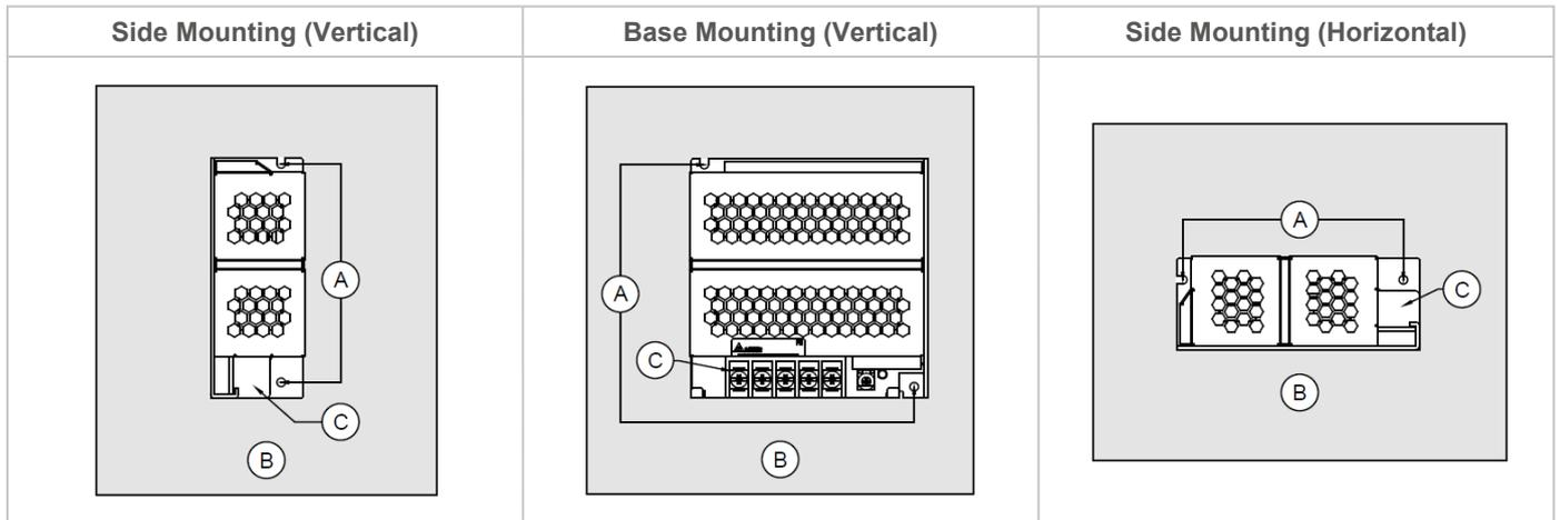
Fig. 2 Mounting Orientation
