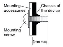
Fig. 4 Mounting Screw
