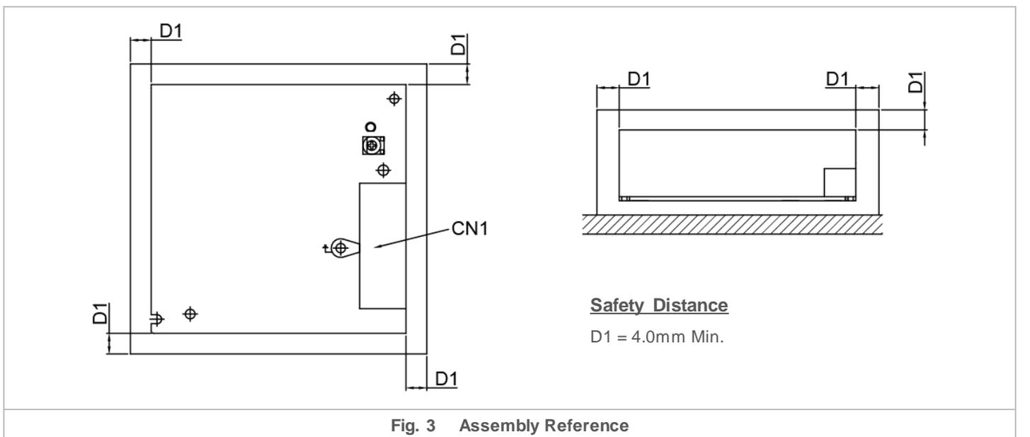
Ensure the mounted device is kept at  $\geq 4\text{ mm}$  (0.16 inch) safety distance at all sides from other components and equipments. In addition, to ensure sufficient convection cooling, always maintain a distance of  $\geq 20\text{ mm}$  (0.79 inch) from ventilated surfaces while the device is in operation.
