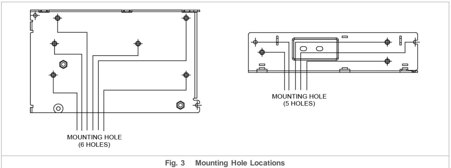
With reference to Fig. 3, the device should be mounted on a sturdy heat conducting surface with minimum of 4 mounting holes using M3 screw through the base or side mounting holes.
