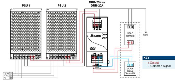
Fig. 5 Redundancy Operation Connection Diagram
