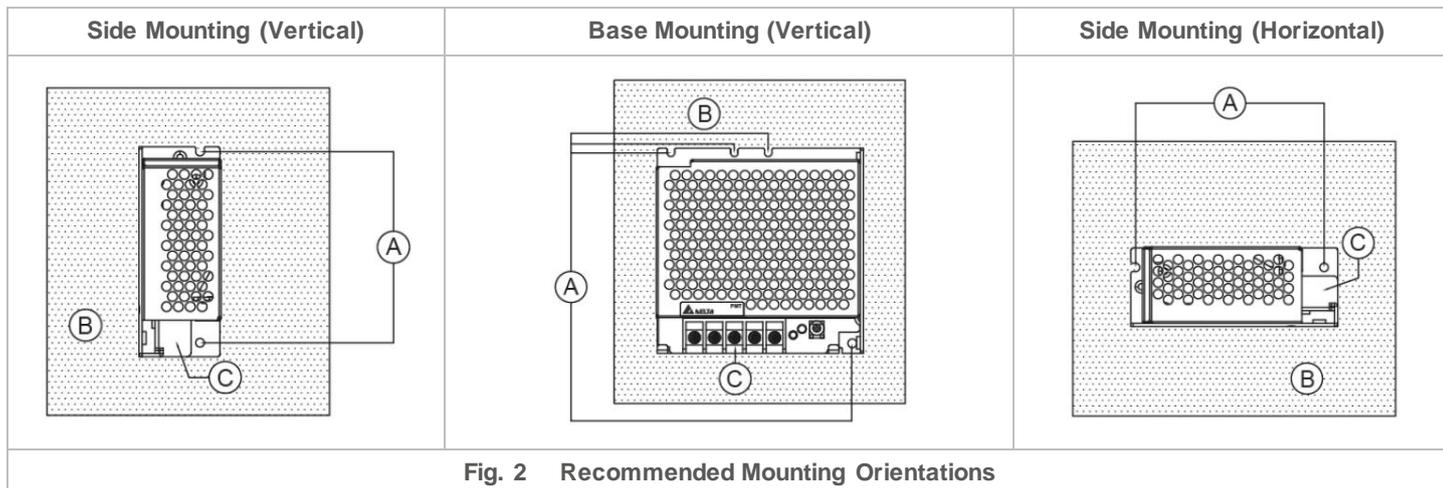
Ensure the mounted device is kept at  $\geq 4$  mm (0.16 inch) safety distance at all sides from other components and equipments. In addition, to ensure sufficient convection cooling, always maintain a distance of  $\geq 20$  mm (0.79 inch) from ventilated surfaces while the device is in operation.
