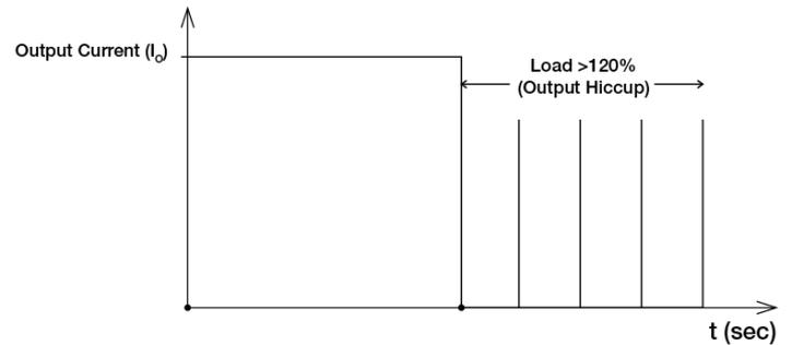
It is not recommended to prolong the duration of  $I_o$  when it is  $<120\%$  but  $>100\%$ , since it may cause damage to the PSU.
