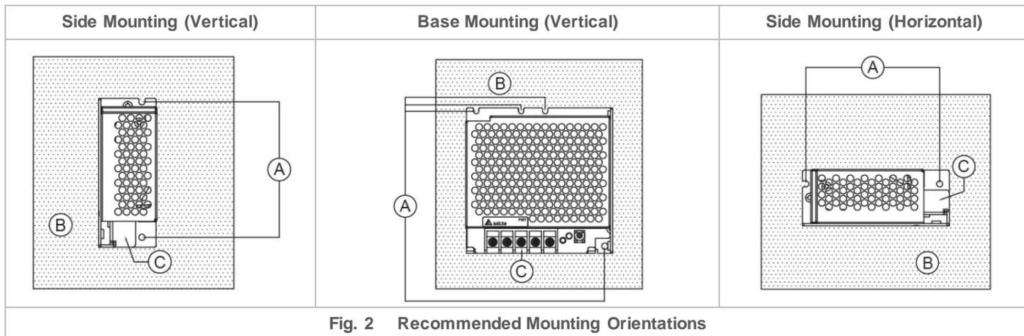
Fig. 2 Recommended Mounting Orientations
