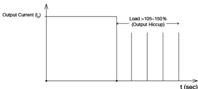
It is not recommended to prolong the duration of  $I_o$  when it is 105%~150%, since it may cause damage to the PSU.
