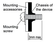
Fig. 4 Mounting Screw
