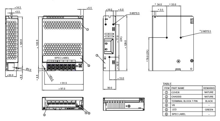
UNLESS OTHERWISE SPECIFIED TOLERANCE OF DIMENSION ARE  $\pm 0.5$ .
