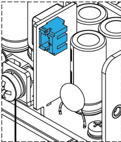
Fig. 9: 12V DC Output Connector (CN801)
