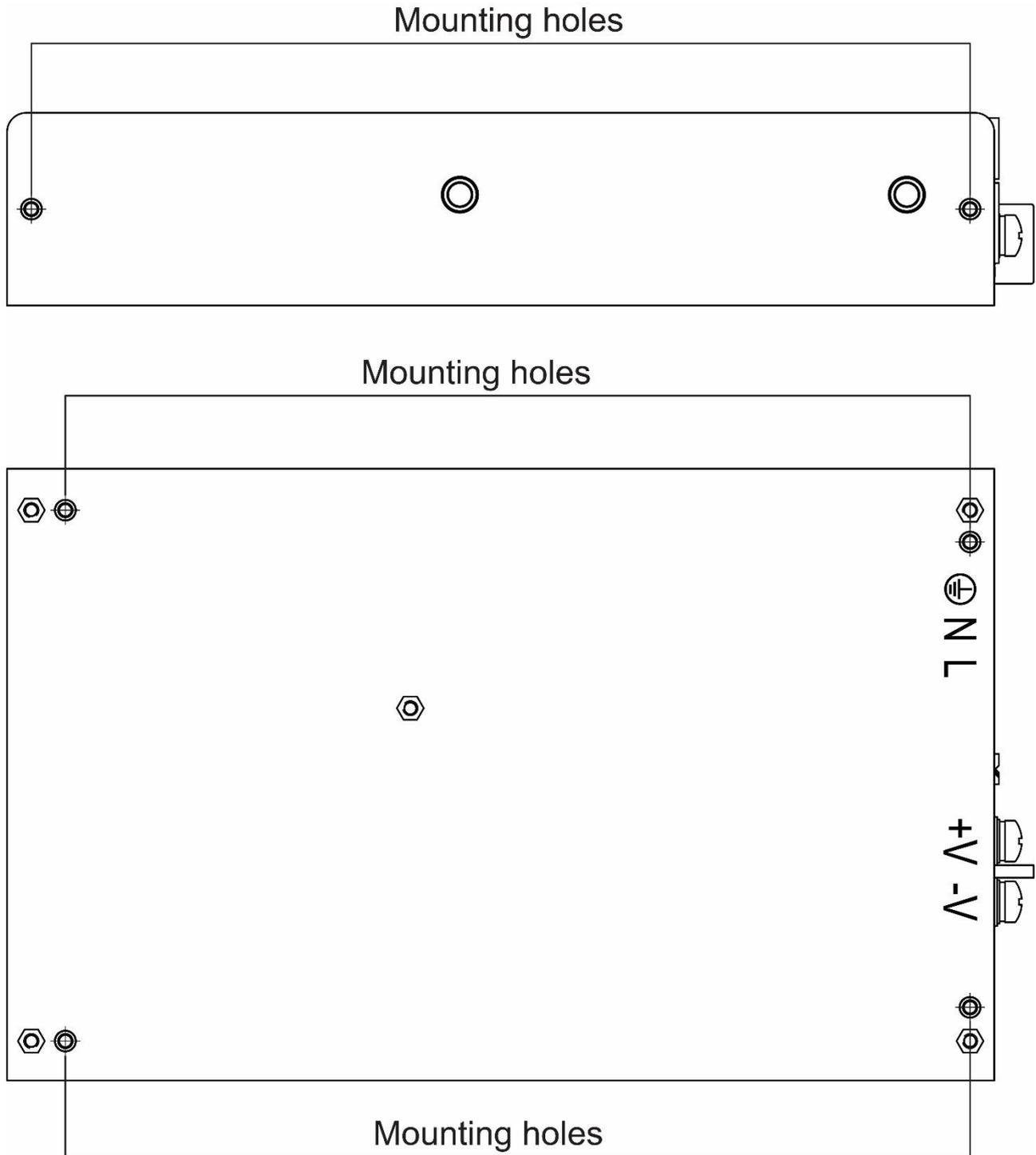
Fig. 15: Position of mounting holes
