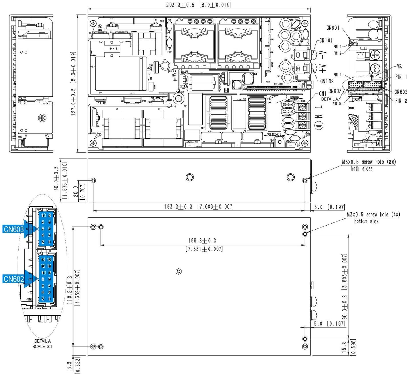
Fig. 16: Dimensional drawing MEU-600C
