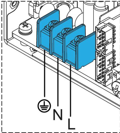
Fig. 2: AC/DC Input terminal block (CN1) – pin assignment
