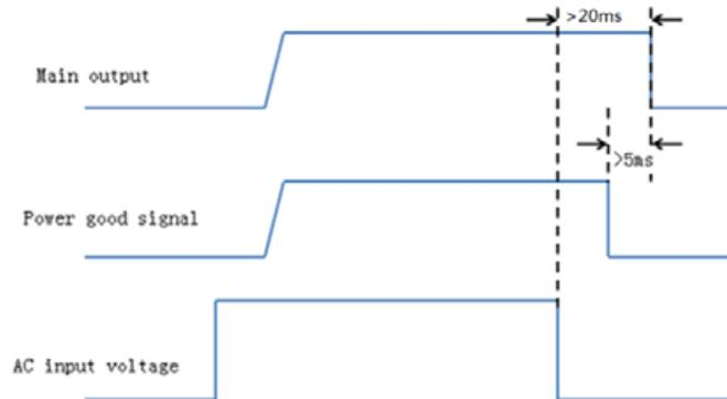
Fig. 24: Power good signal sequence
