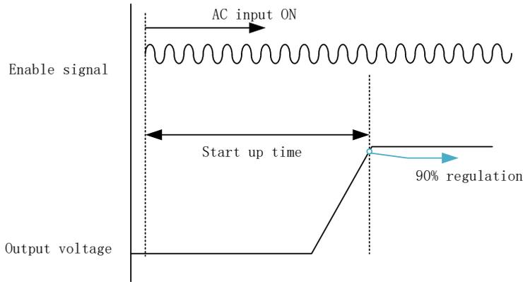
Fig. 17: Start-up timing sequence
