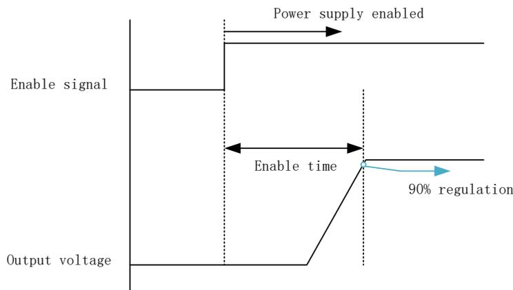
Fig. 18: Enable timing sequence
