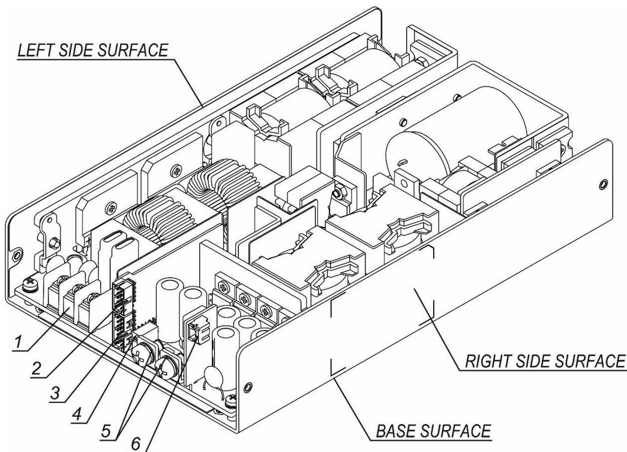
Fig.1: Components of the MEU-600C series
