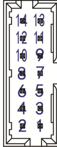
Fig. 5: Signal port and Auxiliary DC Output (CN602)
