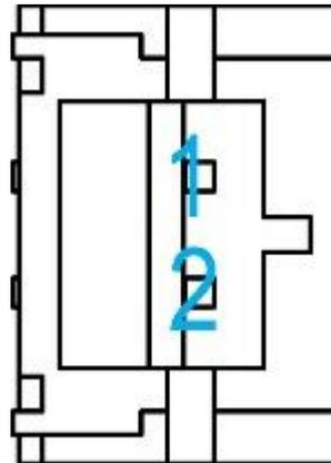
Fig. 10: 12V DC Output Connector(CN801) – pin assignment
