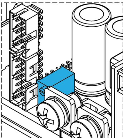
Fig. 7: Output voltage adjustment potentiometer
