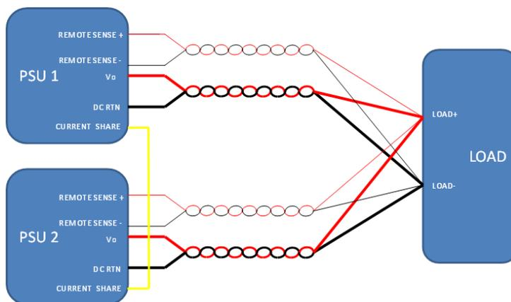
Fig. 26: Parallel connection with remote sense
