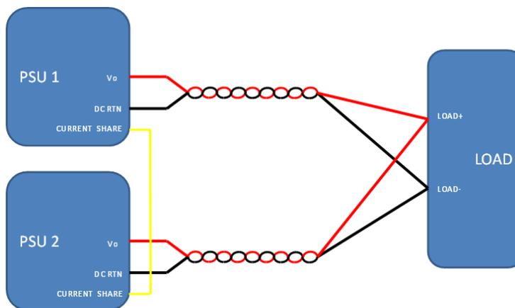
Fig. 27: Parallel connection without remote sense
