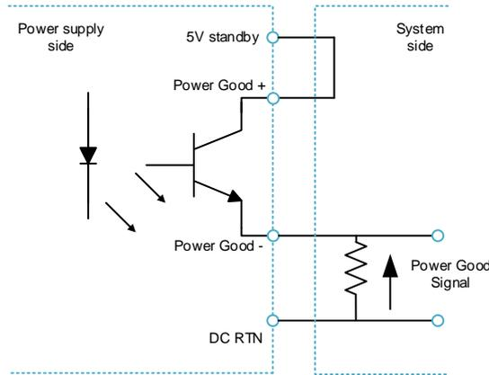
Fig. 23: Power good signal connection
