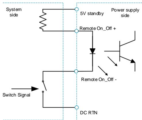
Fig. 22: Remote On\_off connection
