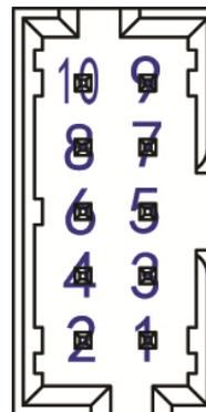
Fig. 4: Signal port and Auxiliary DC Output (CN603)
