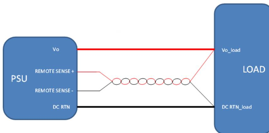
Fig. 25: Remote sense connection
