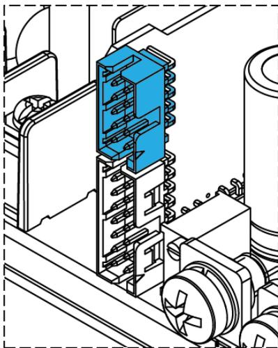
Fig. 3: Signal port and Auxiliary DC Output (CN603)
